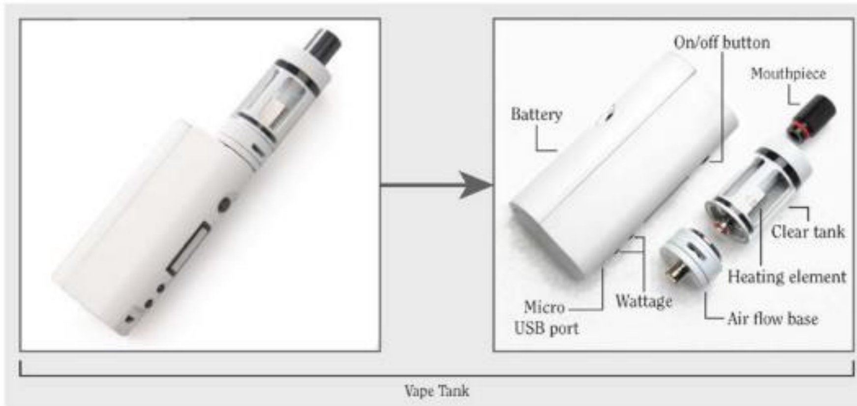
Figure 1.2 Parts of an e-cigarette device
